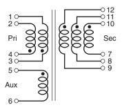
The primary windings and the secondary windings are to be connected in parallel on the PC board.
