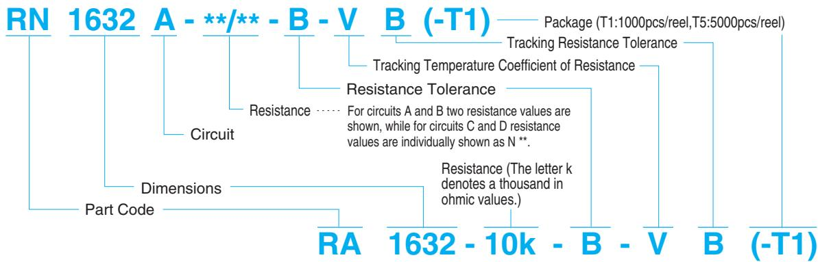
· The specification of a different resistance value or a specific-purpose circuit will assign an individual part code.
