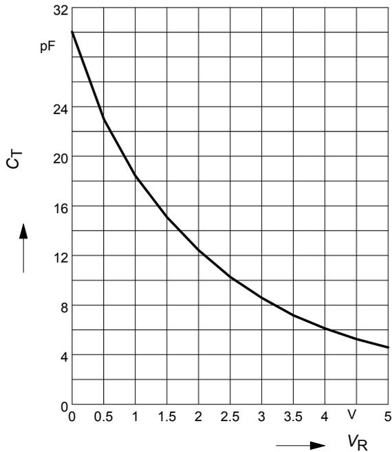
**Normalized diode capacitance**
