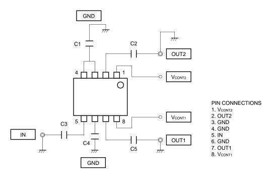
C1, C4 = 10 pF below: Grounding capacitor C2, C3, C5 = 100 pF: DC blocking capacitor
