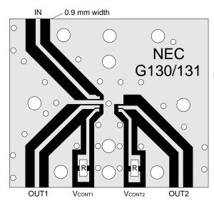
$\begin{pmatrix} 0.4 \text{ mm} \\ \text{thickness} \\ \text{teflon glass} \end{pmatrix}$   $R = 50 \Omega$
