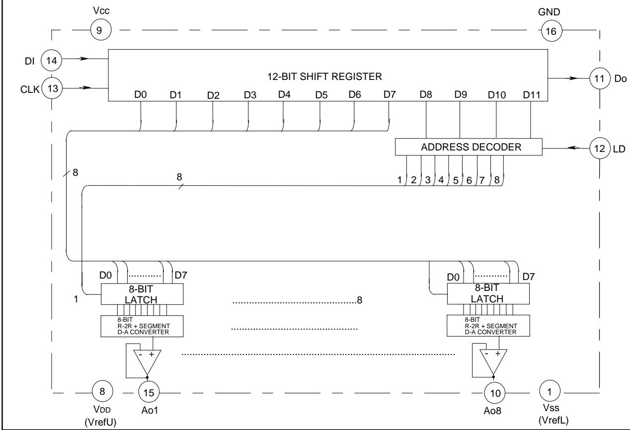
**M62367GP****3V TYPE 8-BIT 8CH D-A CONVERTER WITH BUFFER AMPLIFIERS****DIGITAL DATA FORMAT**LAST
