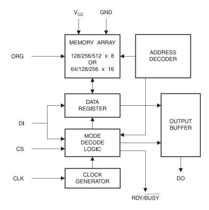
Note: 1. When the ORG pin is connected to V<sub>CC</sub>, the x 16 organization is selected. When it is connected to ground, the x 8 organization is selected. If the ORG pin is left unconnected, then an internal pullup device will select the x 16 organization.
