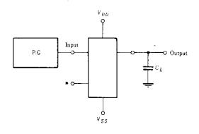
\* All unused inputs of AND, NAND gates must be connected to  $V_{BB}$ .
