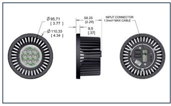
Diameter x H 110.33mm x 58.25mm (4.34" x 2.29") Maximum Cable Dia - 1.5mm<sup>2</sup> / 16 AWG
