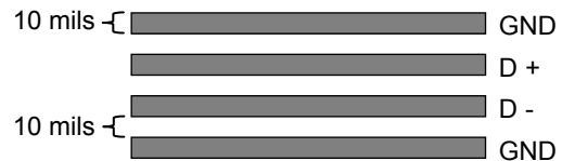
Figure 13 Recommended Remote Diode Circuit Board Interconnect
