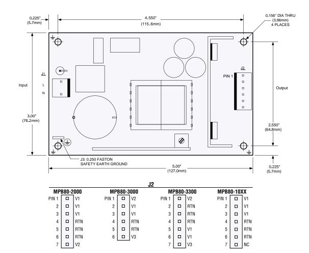
INPUT CONNECTIONS, J1: MOLEX 26-60-4030 OR EQUIVALENT HEADER MATES WITH MOLEX HOUSING 09-50-3031 OR EQUIVALENT AND PINS 08-50-0106 (18-20 AWG) OR 08-50-0108 (22-26 AWG) OR EQUIVALENT.
