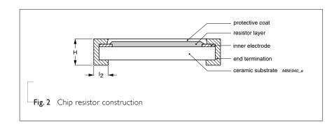
Finally, the two external terminations (pure Tin) are added. See fig. 2.
