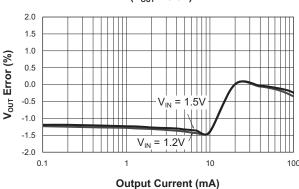
Dual-Cell Load Regulation (V<sub>OUT</sub> = 3.3V)
