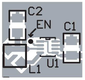
Figure 2: Component Placement.
