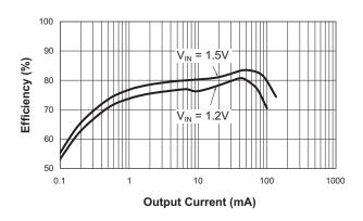
**Dual-Cell to 3.3V Efficiency**
