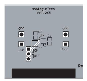
Figure 3: AAT1265 Evaluation Board Bottom Side.
