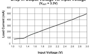
Maximum Load Current Capability for a 4% Drop in Output Voltage vs. Input Voltage
