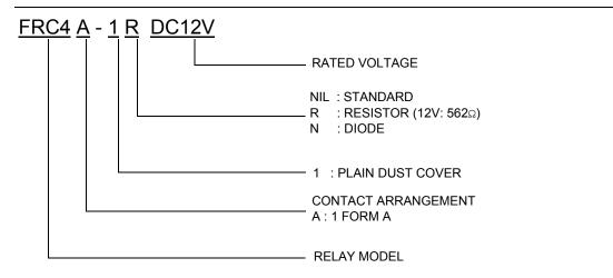
Note: Pb-Free and RoHS compliant relays are available. For ordering, please add suffix "Pb-Free" or "RoHS" to standard relay part numbers.
