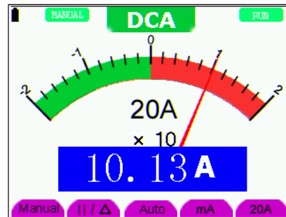
Figure 28: DC Current Measurement.
