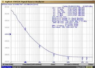
Phase noise of the reference signal, Out3. 25MHz Reference Frequency
