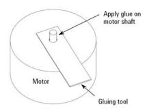
The use of gluing tool is highly recommended. Insert the tool into motor shaft and apply glue around the shaft as shown below. This will help to control the glue thickness. The tool will scrape the excess glue as it is being removed from motor shaft. This will prevent the glue from overflowing into motor or encoder bearing as the motor shaft is inserted into encoder.
