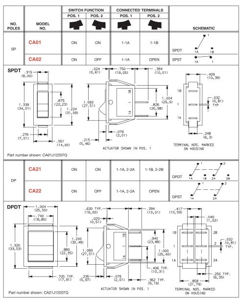
For complete contact ratings and agency approvals, see CONTACT MATERIAL section, page H–111. Contacts make one contact actuator thrown.
