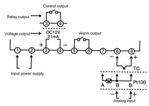
Two input power supplies are available: 100 to 240 VAC or 24 VAC/VDC (no polarity).
