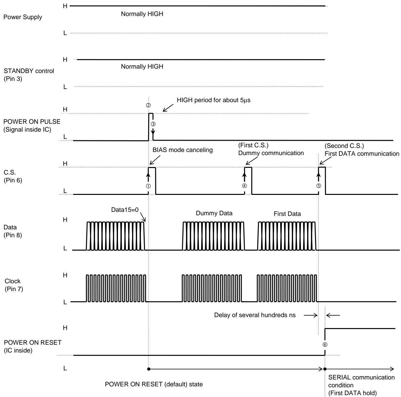
The POWER ON RESET state from the BIAS MODE covers the period from the rise of C.S. ① for communication of canceling of the BIAS MODE to the second rise ⑤ of CS input after the fall ③ of POWER ON PULSE ② generated inside IC. ④ is the dummy communication.
