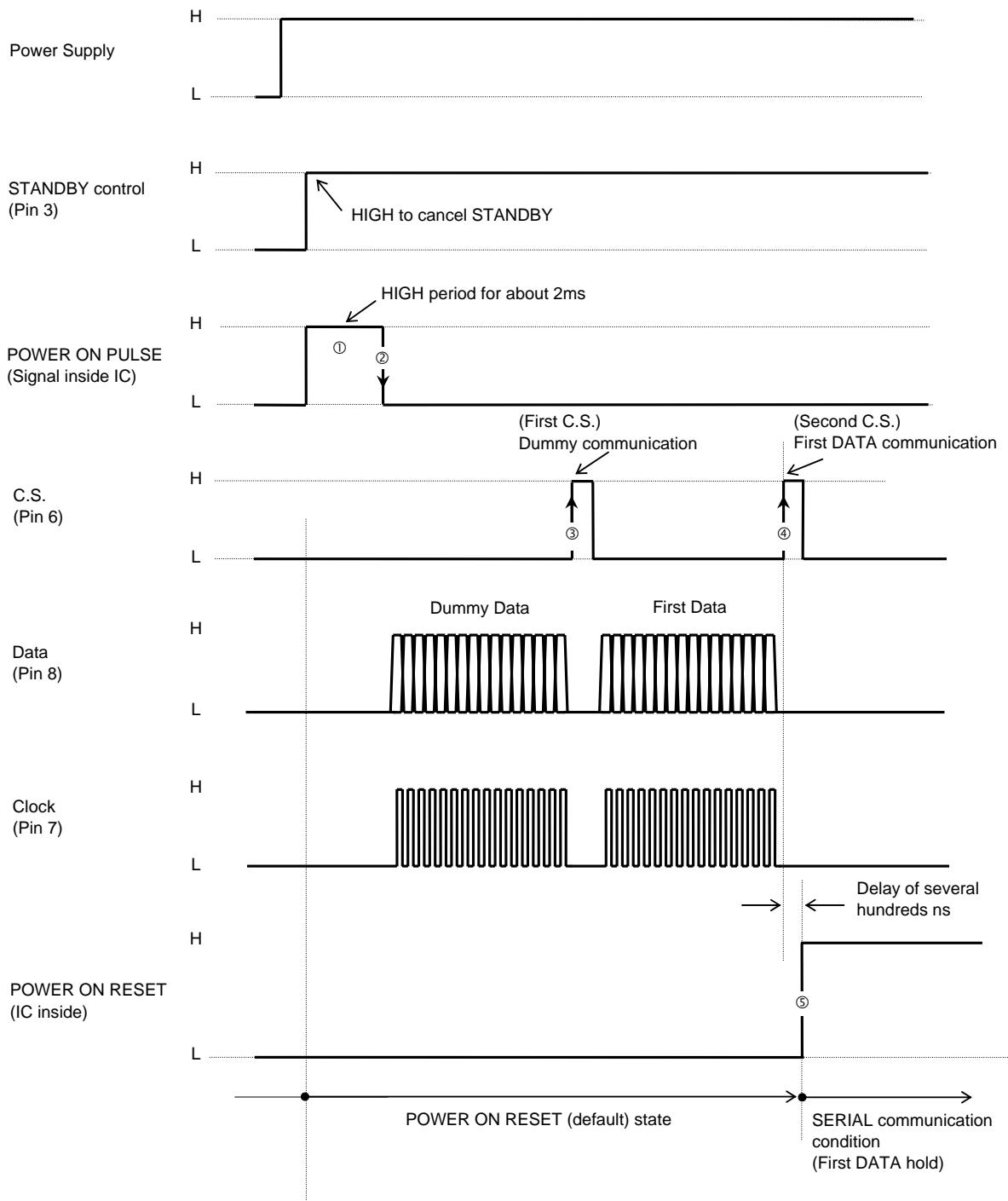
The POWER ON RESET state covers a period up to the rise ④ of the second C.S. input after fall ② of POWER ON PULSE ① generated inside IC when the power is supplied and the STANDBY control is canceled. ③ is the dummy communication.
