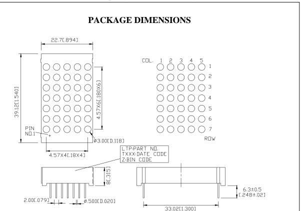
NOTES: 1. All dimensions are in millimeters. Tolerances are  $\pm$  0.25 mm unless otherwise note.
