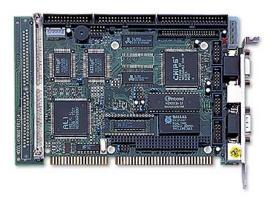
The HS-3000/4M is ISA Bus ALi M6117C chipset industrial single board computer. The board design combine together with all necessary input and output effects interfaces which makes it an ideal all-in-one industrial single board computer. The board design with 40MHz Bus clock rate architecture. The HS-3000/4M supports one SIMM socket with a max. capacity of 16MB and 4MB RAM onboard.
