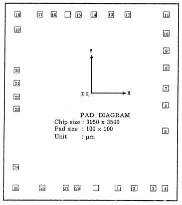
The substrate is connected to VDD.
