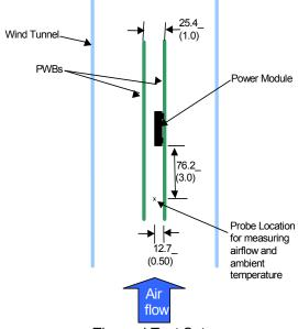
Thermal Test Setup
