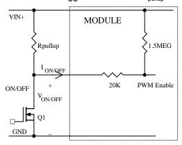
Circuit configuration for using positive On/Off logic
