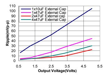
**Note:** Output ripple voltage for various output voltages with external 1x10  $\mu$ F, 1x47  $\mu$ F, 2x47  $\mu$ F or 4x47  $\mu$ F ceramic capacitors at the output (3A load). Input voltage is 12V.
