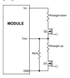
Circuit Configuration for margining Output voltage
