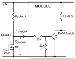
Circuit configuration for using negative On/Off logic
