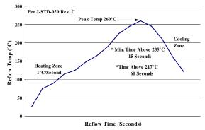
Recommended linear reflow profile using Sn/Ag/Cu solder.
