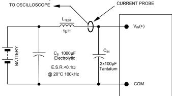
NOTE: Measure input reflected ripple current with a simulated source inductance ( $L_{TEST}$ ) of  $1\mu H$ . Capacitor  $C_S$  offsets possible battery impedance. Measure current as shown above.
