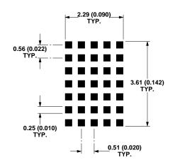
NOTES: 1. UNLESS OTHERWISE SPECIFIED, THE TOLERANCE ON ALL DIMENSIONS IS ± 0.254 mm (0.010"). 2. DIMENSIONS ARE IN MILLIMETERS (INCHES).
