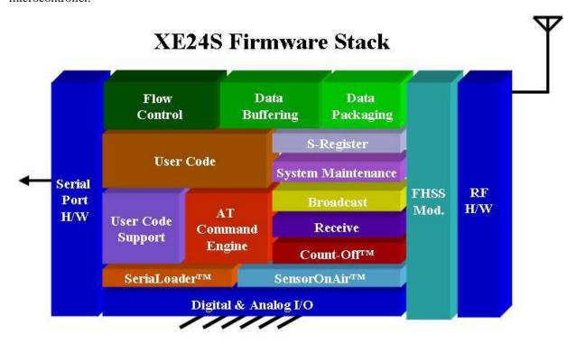
Has shown in the software block diagram above, the User Code interfaces to the rest of the XE24S code through the User Code Support block. The User Code Support block interfaces to the AT command engine and serial interface and supports other features such as sub routine calls.
