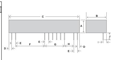
Pin Size: 0.025" by 0.025" Recommended hole size: 0.056" All pins tin-plated.
