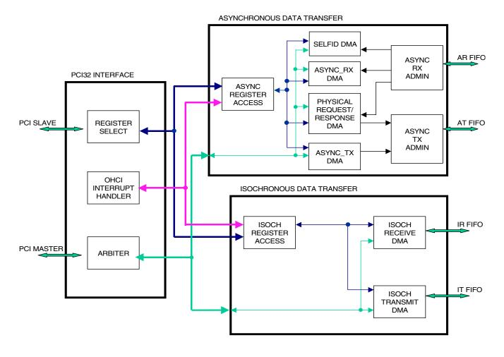
Figure 3. OHCI Core Block Diagram
