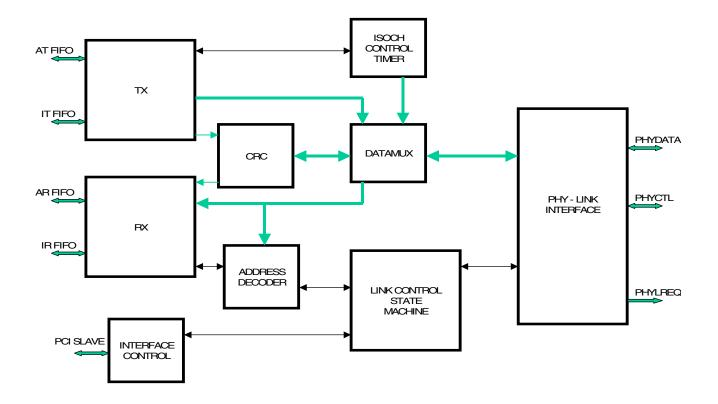
Figure 4. Link Core Block Diagram
