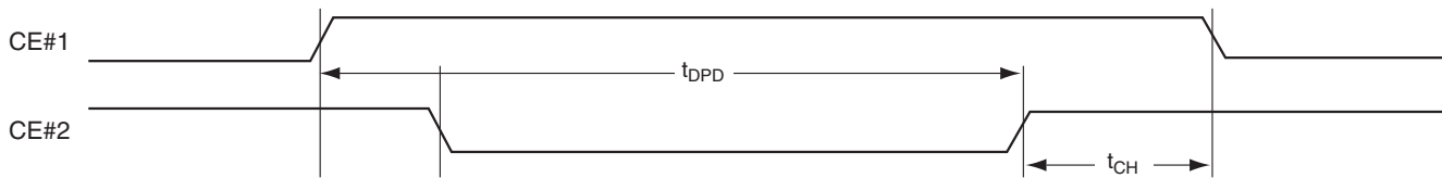
Figure 33. Deep Power-down Timing
