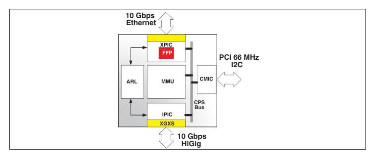
The BCM5673 10 Gigabit Ethernet switch is a scalable, multi-layer switch-on-chip member of the StrataXGS family. The BCM5673 is a dual port switch, which supports a 10 Gigabit Ethernet (IEEE802.3ae) port and a HiGig™ uplink port. The 10 Gigabit Ethernet port can be used to interface to the XENPAK module via the XAUI interface.
