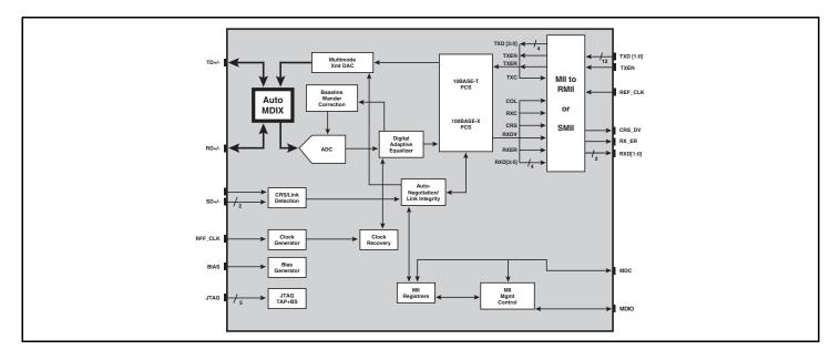
The Broadcom® BCM5226 is a single-chip device containing six independent Fast Ethernet transceivers. Each performs all the physical layer interface functions for 100BASE-TX full-duplex or half-duplex Ethernet on Category 5 twisted-pair cable and 10BASE-T full or half-duplex Ethernet on Category 3, 4 or 5 cable. Each port may also be configured for 100BASE-FX full or half-duplex transmission over fiber-optic cabling when paired with an external fiber-optic line transceiver.
