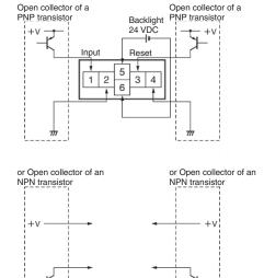
Note: 1. Terminals 2 and 4 (input circuit and reset circuit) are functionally isolated.
