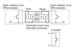
Note: 1. Residual voltage in the output section of Proximity Sensors or Photoelectric Sensors becomes less than 0.5 V because the current flowing from terminals 1 or 3 is as small as approx. 10 µA, thus allowing easy connection.
