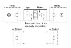
Note: Use Relays and Switches that have high contact reliability because the current flowing from terminals 1 or 3 is as small as approx. 10 µA. It is recommended that OMRON's G3TA-IA/ID be used as the SSR.
