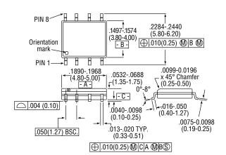
8- Lead SOP outline dimensions Narrow body .150 (All dimensions per JEDEC No. MS-012-AA, Issue C) Dimensions in ( ) are in mm.
