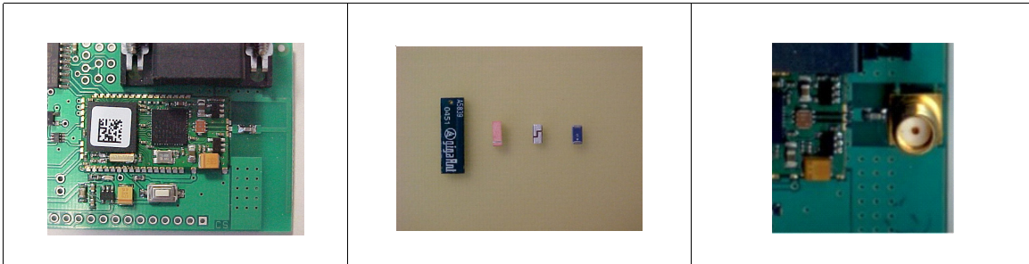
Figure 5. SMA connector for external antenna
