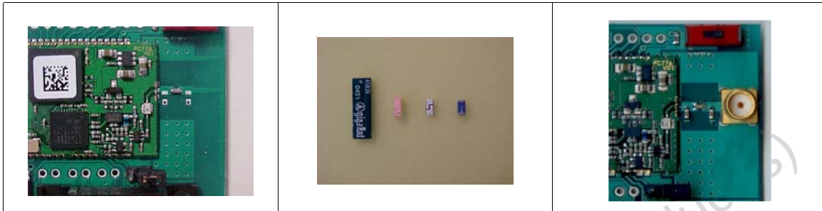
Figure 5. SMA connector for external antenna
