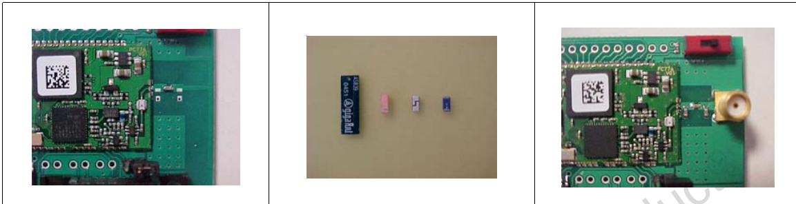
Figure 5. SMA connector for external antenna
