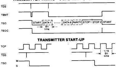
Upon data transmission initiation, or when not transmitting at 100% line utilization, the start bit will be placed on the TSO line at the high to low transition of the TCP clock following the trailing edge of  $\overline{\text{TDS}}$ .
