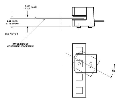
For linear motion, angular misalignment, E  $_{\rm A}$ , must be  $\leq~\pm~2$  degrees to achieve Encoding Characteristics.
