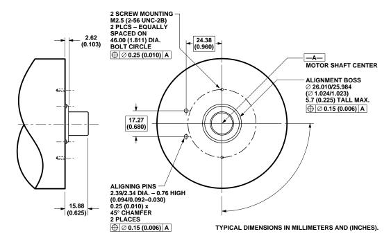
If neither locating pins nor locating boss are available, then a centering tool supplied by Agilent can be used (HEDS-6510).
