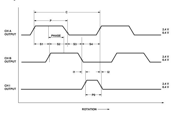
**Waveforms for Encoders without Line Drivers.**
