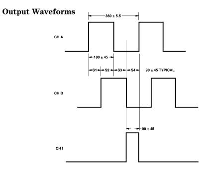
NOTE: ALL VALUES ARE IN ELECTRICAL DEGREES, WHERE  $360^\circ$  e = 1 CYCLE OF RESOLUTION. ERRORS ARE WORST CASE OVER ONE REVOLUTION. CH B LEADS CH A FOR COUNTERCLOCKWISE ROTATION. CH A LEADS CH B FOR CLOCKWISE ROTATION.
