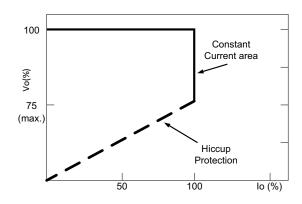
Typical LED power supply I-V curve
