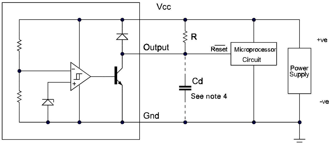
Note 4: A time delayed reset can be accomplished with the additional  $C_d$ .
