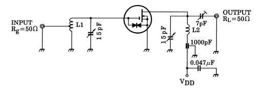
L1: 1.0 mm $\phi$  silver plated copper wire 4.0 T, 8 mm $\phi$  ID TAP at 1.0 T from coil end
