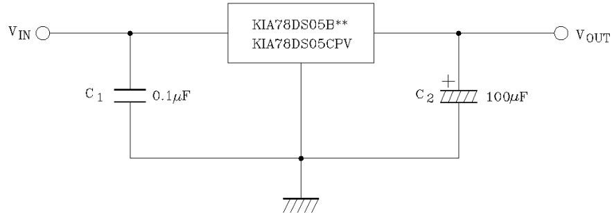
Capacitor  $C_2$  must be guaranteed to operate in the temperature range that the regulator should be operated correctly,  $100\mu F$  is a suitable value to suppress the oscillation phenomenon at the output terminal.
