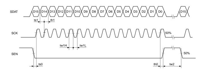
Fig. 3. Serial transfer block measurement conditions
