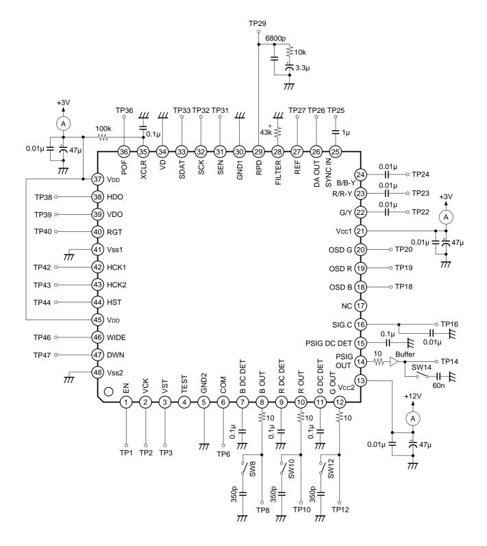
\* Resistance value tolerance: ±2%, temperature coefficient: ±200ppm/°C or less Locate this resistor as close to the IC pin as possible to reduce the effects of external signals.
