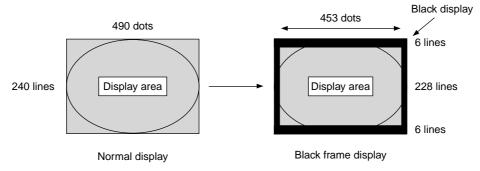
• AC driving of LCD panels during no signal
