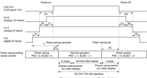
When power saving is set to on or off, video display is automatically turned on or off at the above timings.
