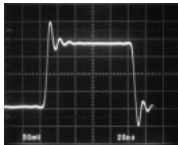
Small-Signal Transient, A_V = 1
