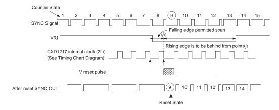
Since the falling edge point in the diagram above (marked with  $\uparrow$ ) is the boundary of reset, if the falling edge of the VRI input traverses that point, it causes 1/2H deviation to the reset state.
