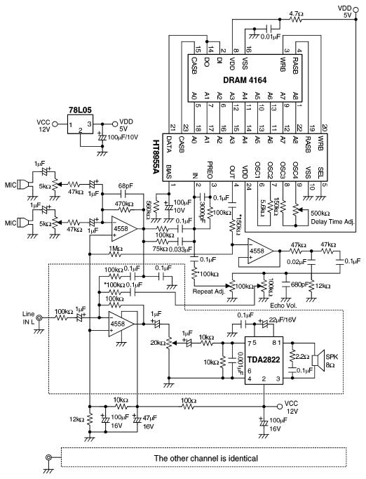
\*Note: In practical applications, the value of the marked part may be adjusted to the desired effect
