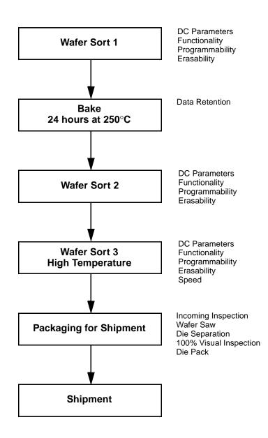
Figure 1. AMD KGD Product Test Flow
