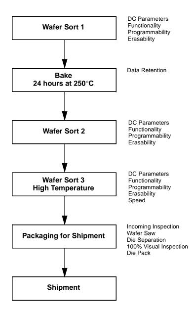
Figure 1. AMD KGD Product Test Flow
