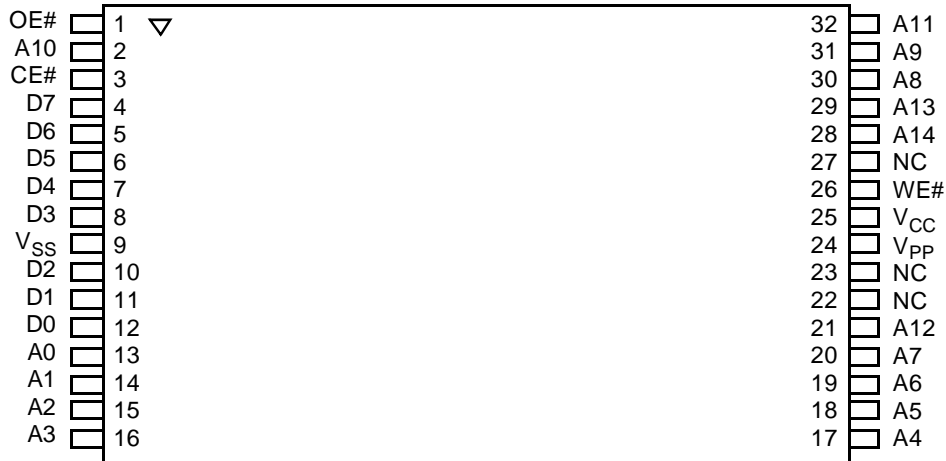
32-Pin TSOP—Reverse Pinout
